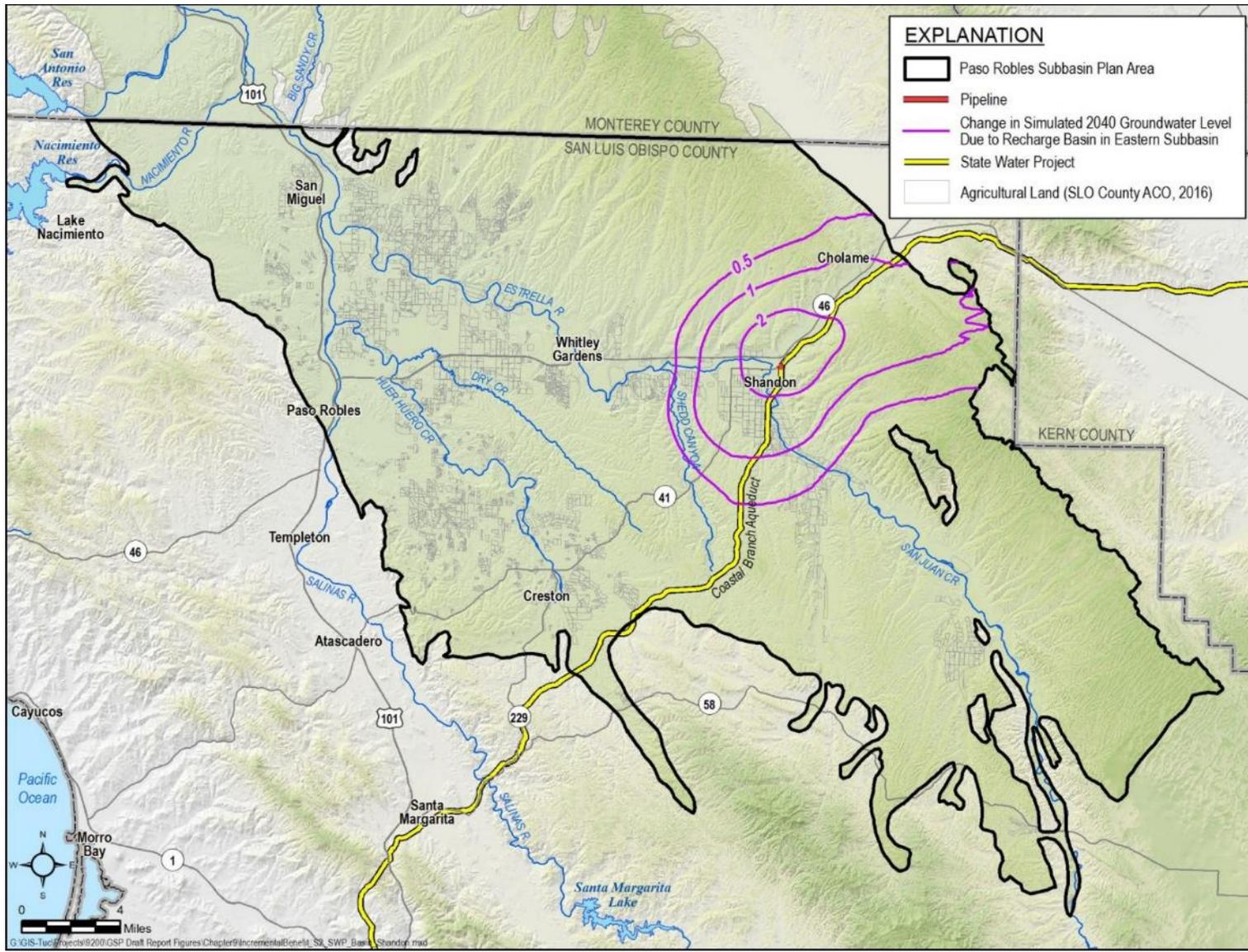
Figure 9-23. Groundwater Level Benefit from Recharge Basin in Eastern Subbasin
