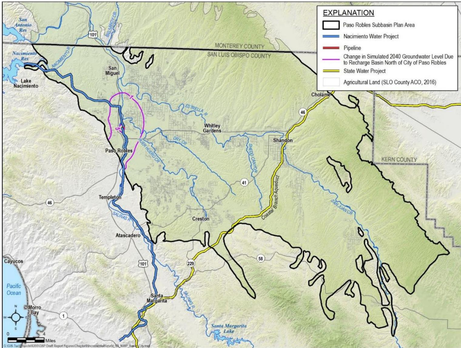
Figure 9-26. Groundwater Level Benefit from Recharge Basin North of City of Paso Robles
