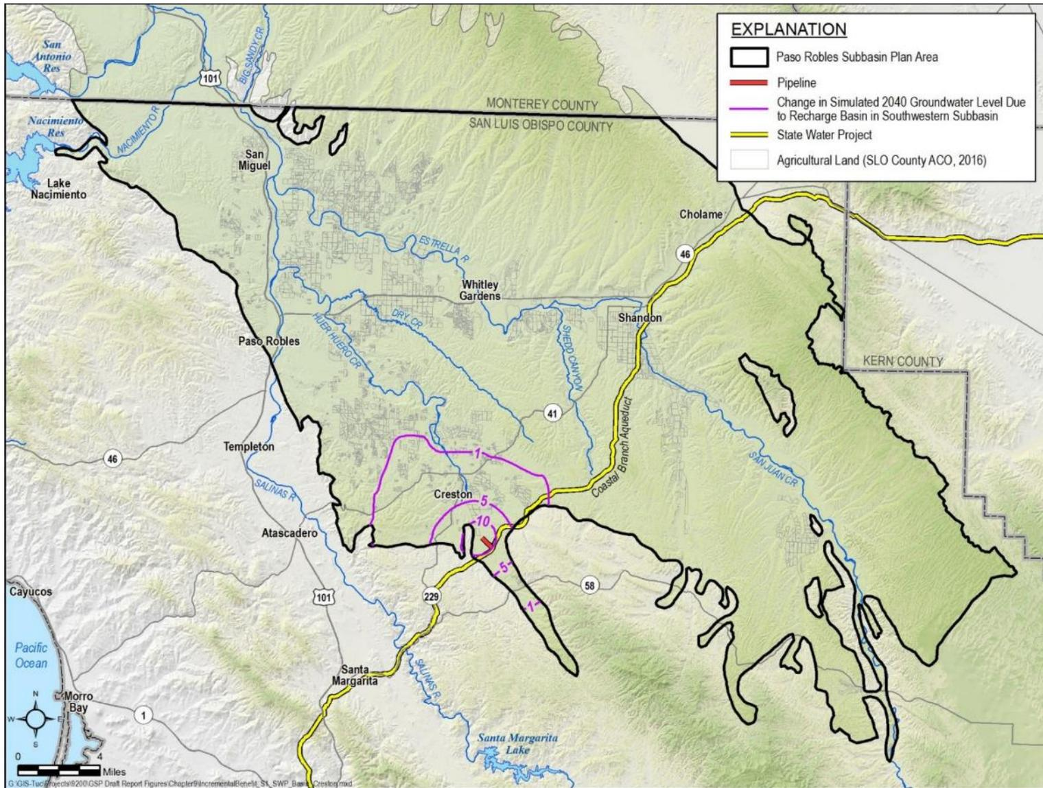
Figure 9-20. Groundwater Level Benefit from Recharge Basin in Southwestern Subbasin
