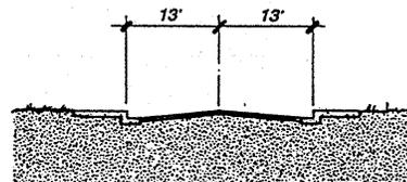
Reduce curb-to-curb street width from 36 to 24 feet for typical 50 ACT to 1500 ADT road section. Best suited to short loop roads where little through traffic can be expected.
