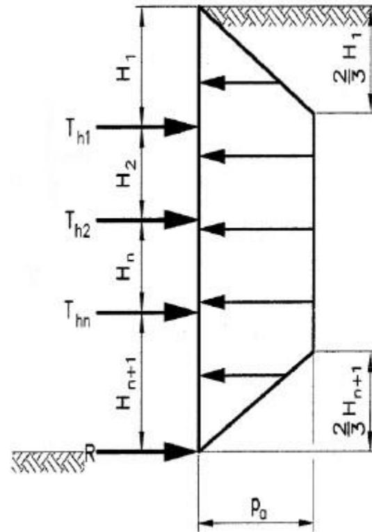
**Figure 6: AEP Distribution for Anchored Walls with More than one Anchor (AASHTO 2017)**
