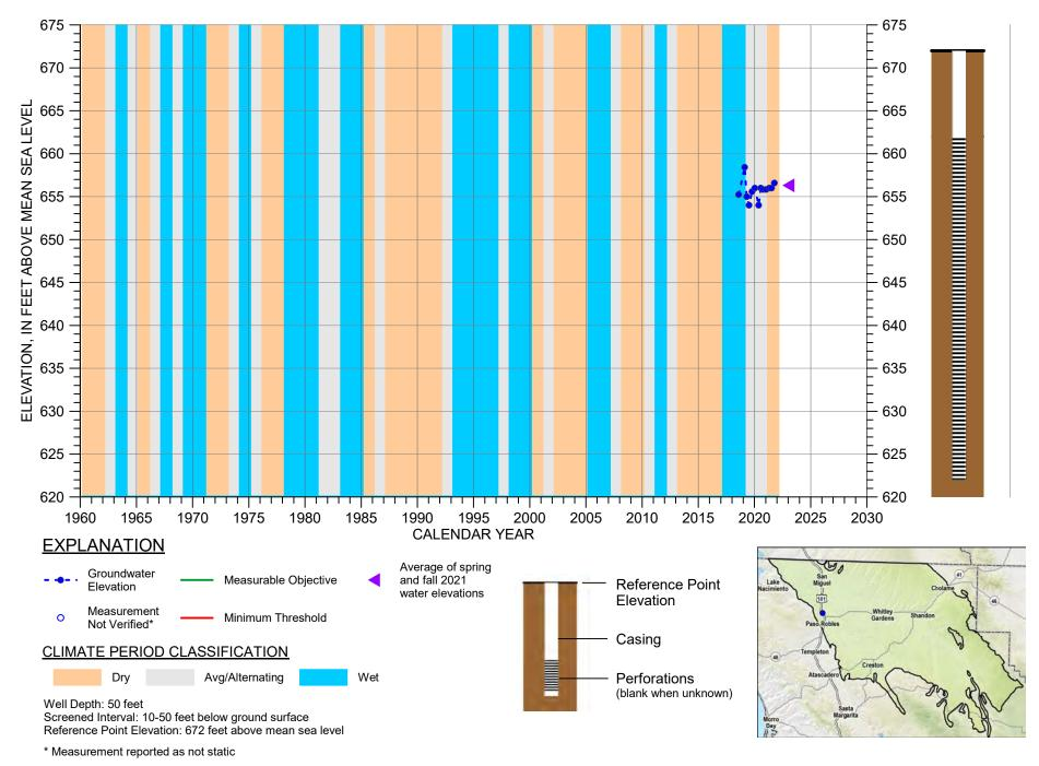
HYDROGRAPH OF MEASURED GROUNDWATER ELEVATION FOR 18MW-0191
