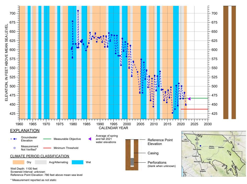
HYDROGRAPH OF MEASURED GROUNDWATER ELEVATION FOR 26S/12E-14K01
