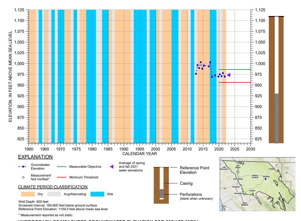
HYDROGRAPH OF MEASURED GROUNDWATER ELEVATION FOR 26S/15E-29R01
