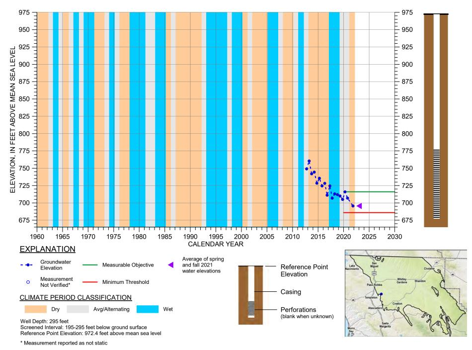
HYDROGRAPH OF MEASURED GROUNDWATER ELEVATION FOR 27S/12E-13N01
