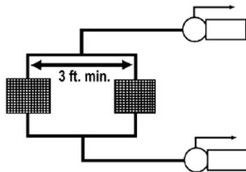
26. Split suction must be plumbed so they are hydraulically balanced. See diagram below.
