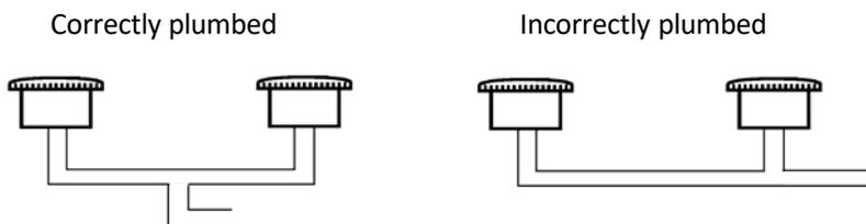
27. A main drain connected directly to a skimmer requires a split main drain.
