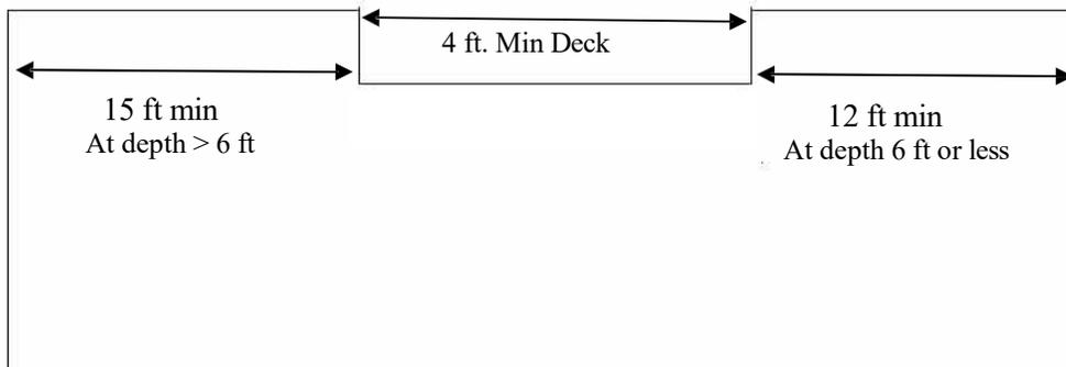
7. For "L" or irregularly shaped pools, the minimum width (12 ft. or 15 ft.), must be maintained for both sections of the "L."
