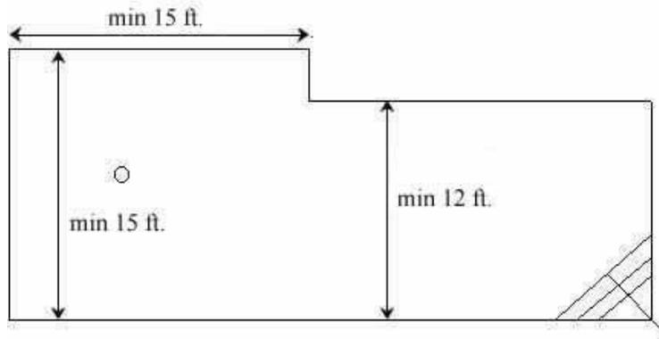
6. No recesses or projections are permitted in swimming pools. An area is not considered a recess or projection, and will be permitted, if it is 12 ft. or more in length in a pool with a maximum depth of 6 feet or less or 15 ft. or more in length in a swimming pool with a maximum depth greater than 6 feet. Swimouts, loveseats, baja steps and foot holds are prohibited.
