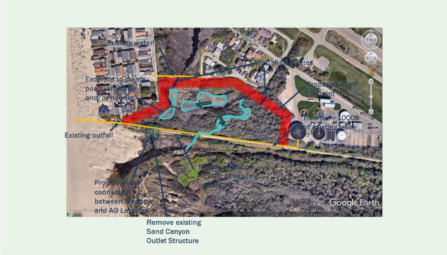
Figure 1. Levee setback alternative showing relocated levee (red) and Sanitation District outfall pipe (yellow) along the south side of Meadow Creek Lagoon.
