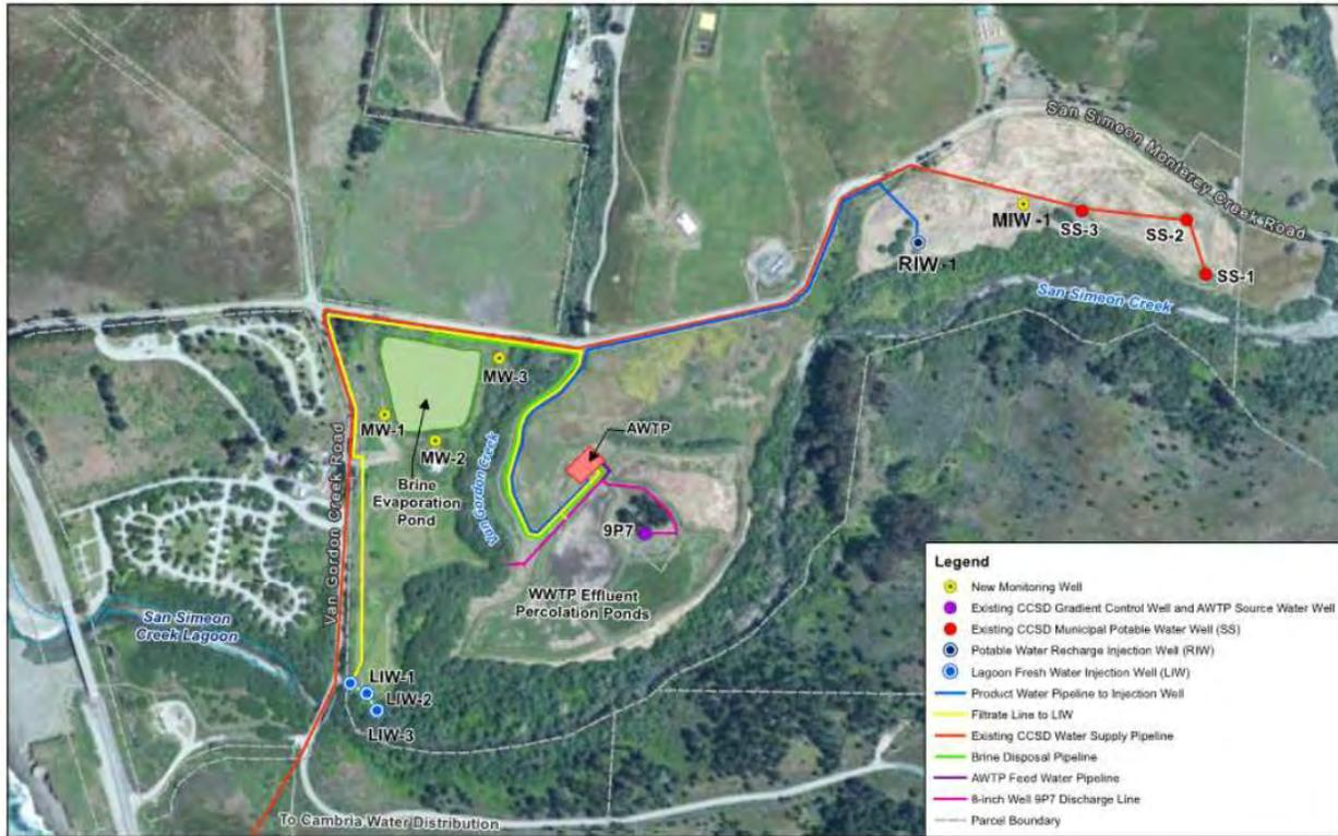
Figure D-4. Cambria CSD Desalination Schematic
