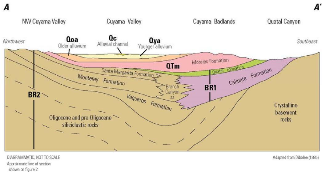
FIGURE 6: Stratigraphic Diagram of the Cuyama Valley Area
