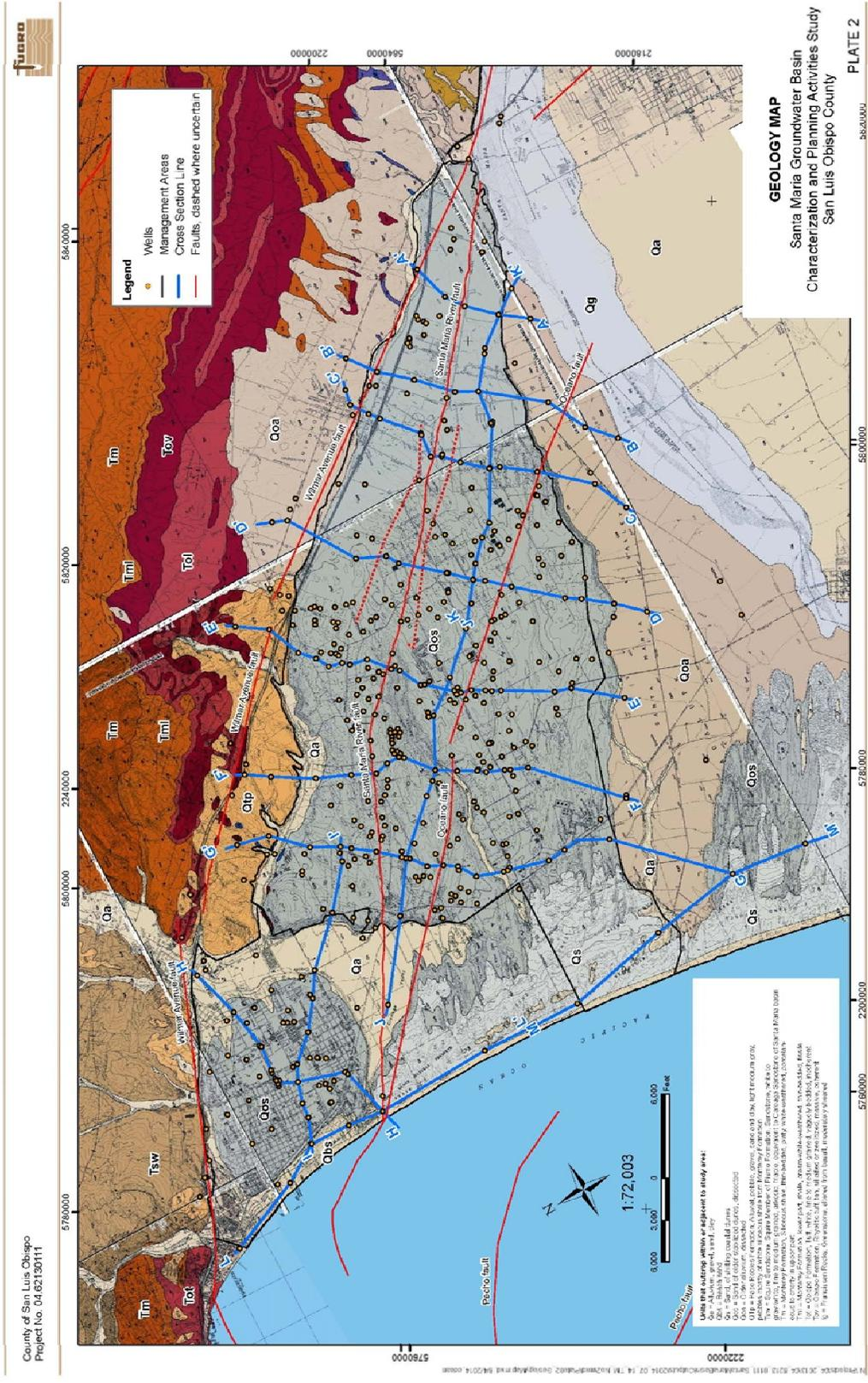
FIGURE 19: Santa Maria Valley Groundwater Basin Geology and Location of Geologic Sections
