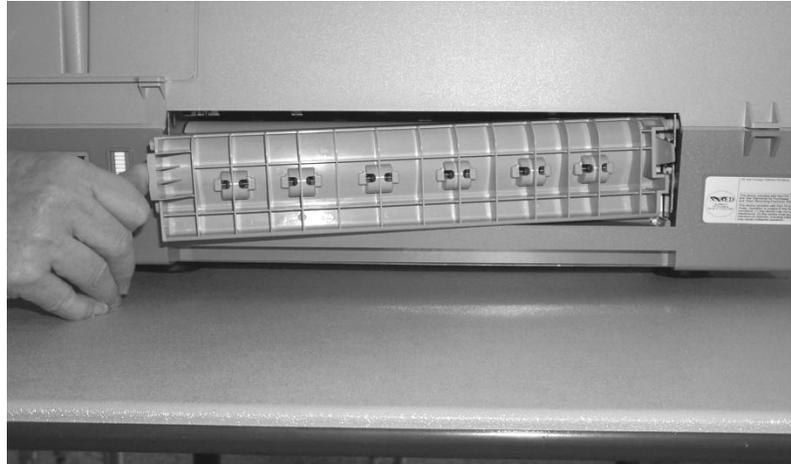
To replace, if necessary, put the two prongs on the tray in the holes on the right. Push tab on the left to the right and push into place.
