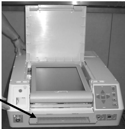
7. Lift the screen to the full upright position. Move back sliding latches behind the screen to prevent it from falling backward.
