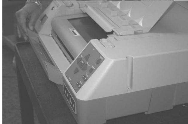
6. Fold down the front flap of the lid. Move sliding latches over the front flap to keep securely closed.
