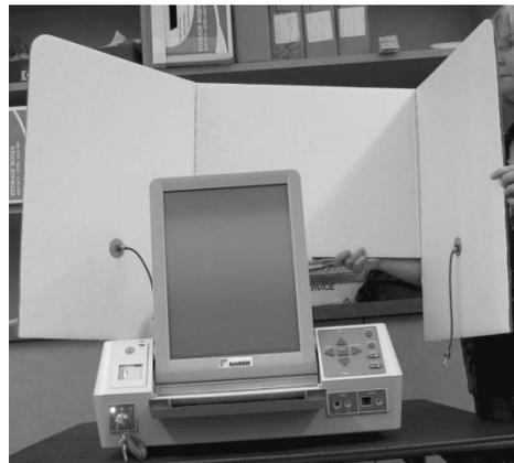
3. Raise the lid, slide the latches and lower the screen to flat position.
