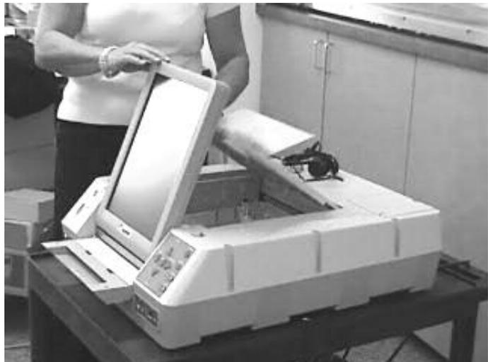
9. Plug headset into the Audio socket to the right, rest on table.
