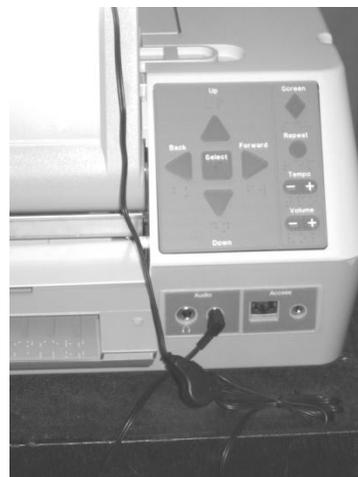
10. Plug Scroll/Select Paddle into the Access socket on the far right side of the Auto MARK.
