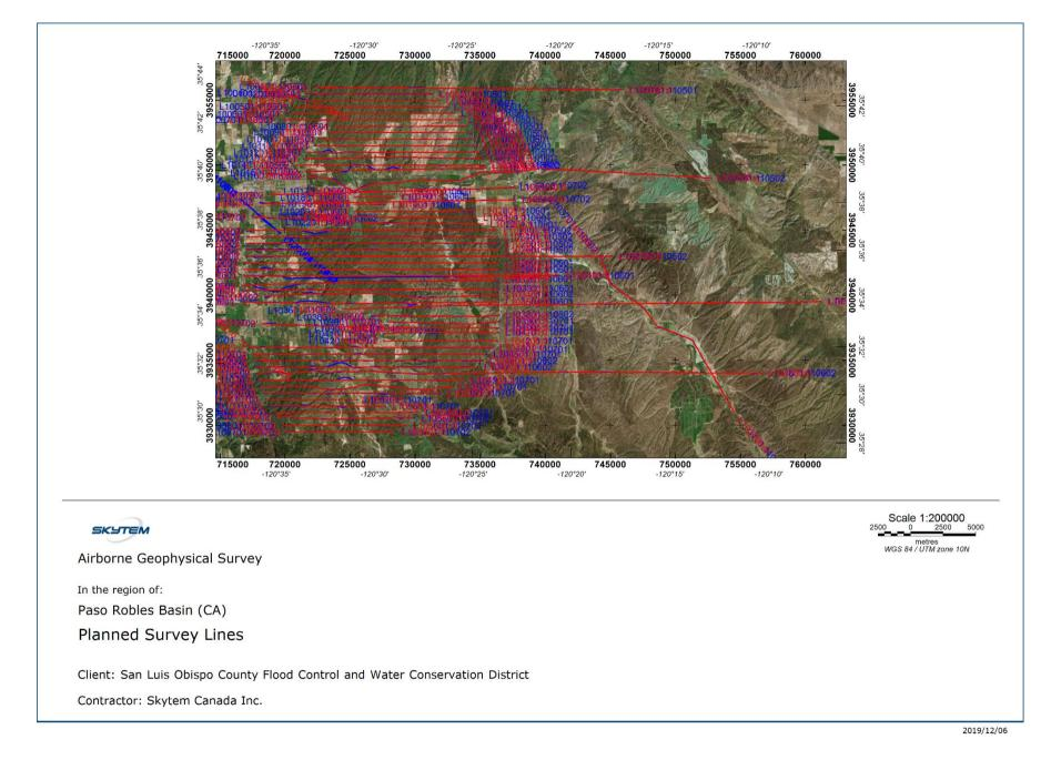
Figure 2: Paso Robles Basin, Flown lines (blue) superimposed on planned lines (red).
