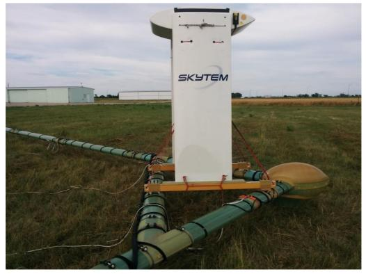
Figure 19: Rudder containing the Z coil located in the top part of the tower.
