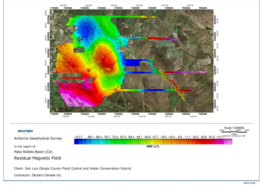
Figure 14: Residual Magnetic Field.
