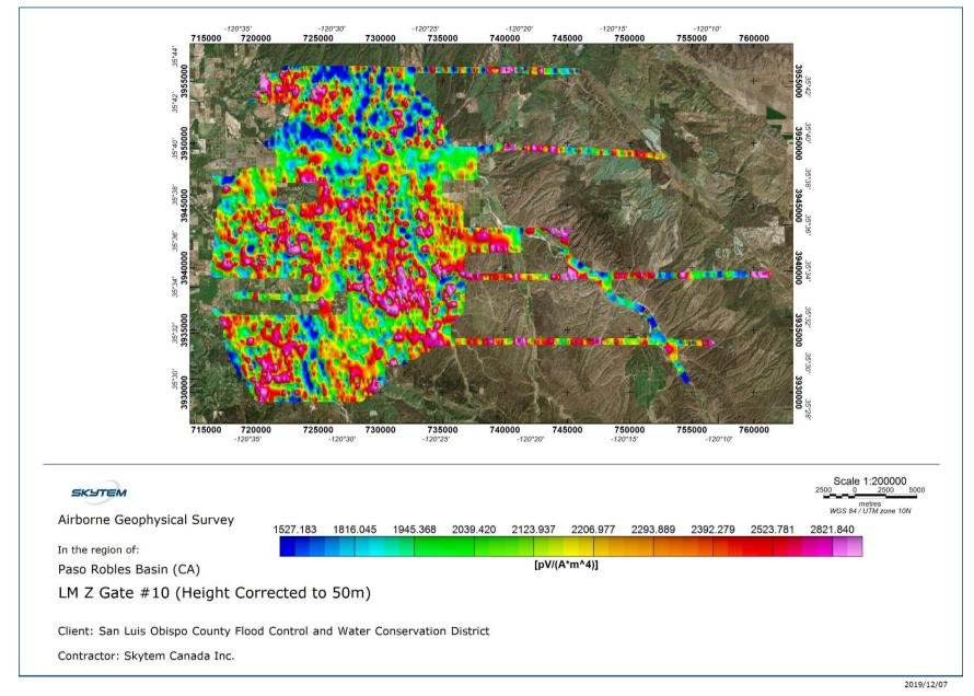
*Figure 15: Low Moment Z coil (gate 10). Warm colors (red) represent high intensity.*
