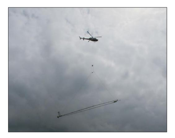
Figure 3: SkyTEM312M Airborne unit.
