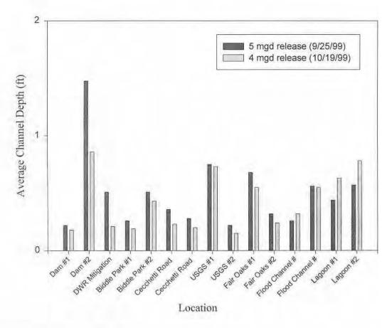
Figure 3-22. Results of transect measurements comparing average channel depth (feet) during experimental streamflow releases from Lopez Dam, September-October 1999.
