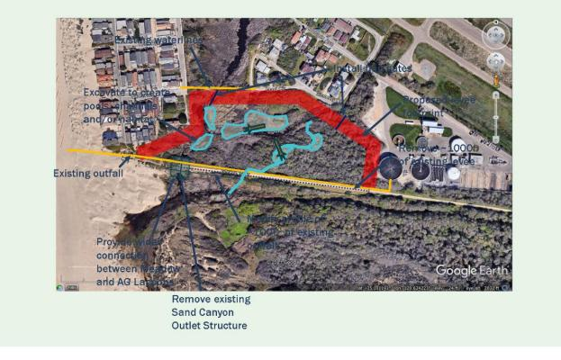
Figure 1. Levee setback alternative showing relocated levee (red) and Sanitation District outfall pipe (yellow) along the south side of Meadow Creek Lagoon.
