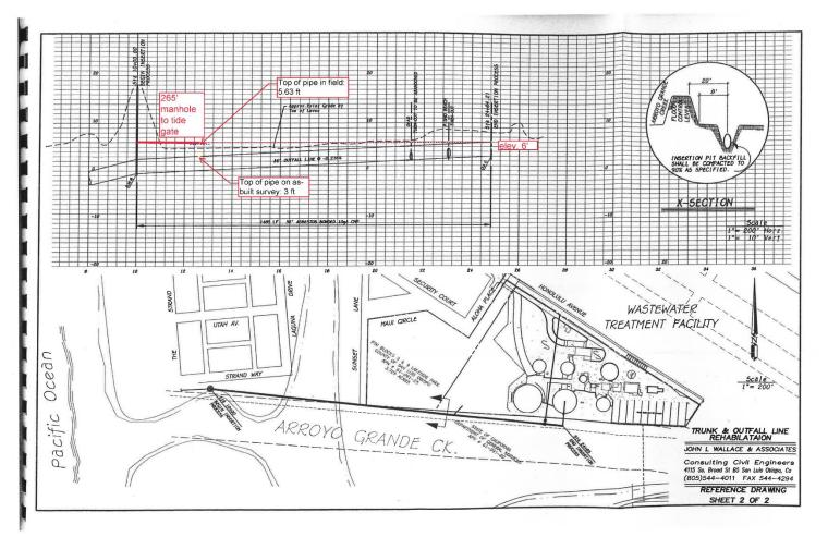
Figure 3. Sanitation District Outfall Pipe 1997 plan for repair (sliplining) of pipe, annotated with District field measurement of depth to pipe near flap gate.
