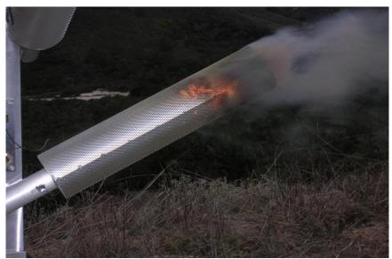
Figure 4.4 Flare burning inside a spark arrestor
