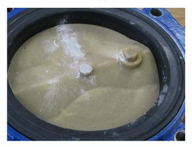
Photo 2: Excessively thick scale layer on the metal surface of a butterfly valve.
