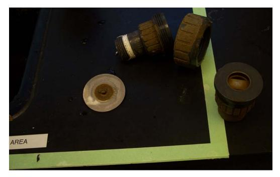
Photo 1: Scale formation plugging the DAF diffuser nozzles
