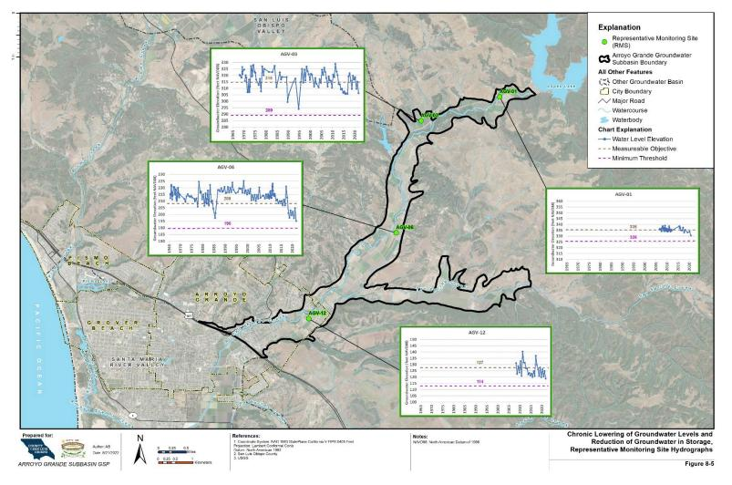
Figure 8-5 Chronic Lowering of Groundwater Levels and Reduction in Groundwater in Storage, Representative Monitoring Site Hydrographs
