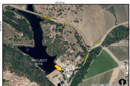
Lopez Water Treatment Plant and its primary distribution line provides the p[rimary water supply to the five cities. The project will install a SCADA system for remote monitoring and control of the pipeline system.
