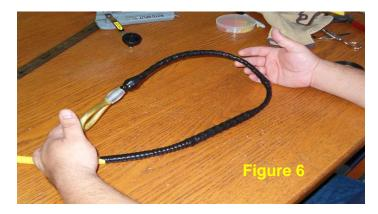
8. Ensure that the tensile load applied to the cable is within the manufacturers recommendations for that product. Ensure the correct size pulling grip is used. Failure to do so may lead to improper coupling of the grip to the cable strength elements and may create the potential for cable damage.
