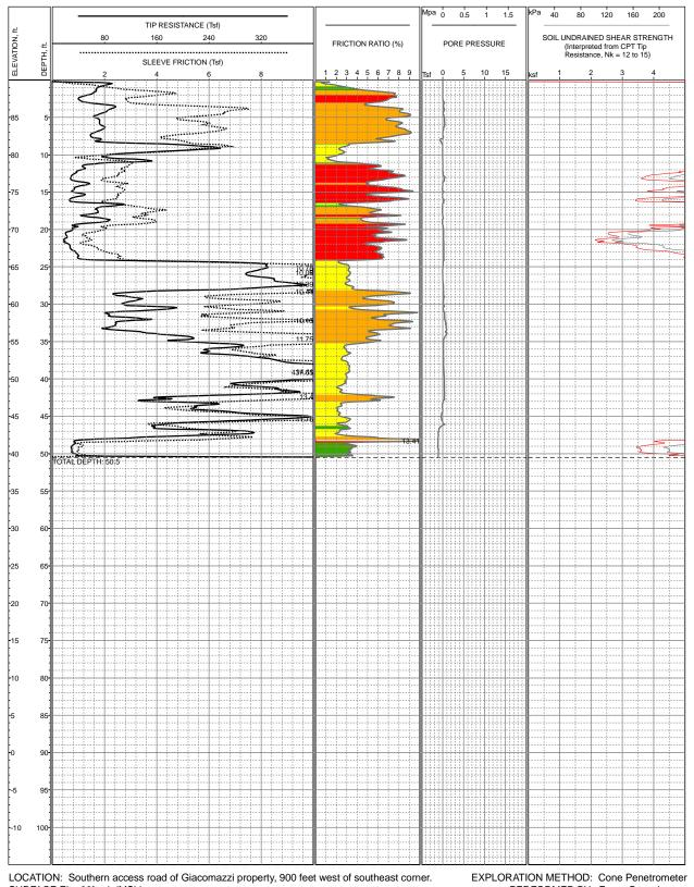
SURFACE EL: 90ft +/- (MSL) COMPLETION DEPTH: 50.5ft TESTDATE: 5/8/2007 EXPLORATION METHOD: Cone Penetrometer PERFORMED BY: Fugro Geosciences REVIEWED BY: J Blanchard
