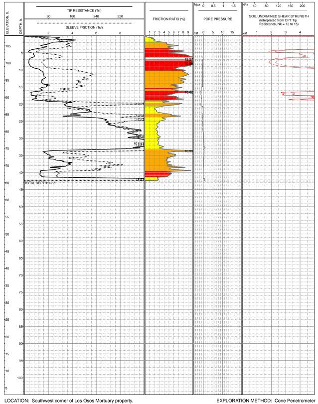
LOCATION: Southwest corner of Los Osos Mortuary prop SURFACE EL: 108ft +/- (MSL) COMPLETION DEPTH: 42.5ft TESTDATE: 5/8/2007 EXPLORATION METHOD: Cone Penetrometer PERFORMED BY: Fugro Geosciences REVIEWED BY: J Blanchard
