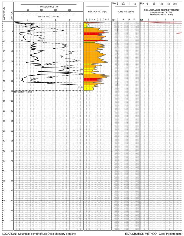
LOCATION: Southeast corner of Los Osos Mortuary prope SURFACE EL: 105ft +/- (MSL) COMPLETION DEPTH: 34.9ft TESTDATE: 5/8/2007 EXPLORATION METHOD: Cone Penetrometer PERFORMED BY: Fugro Geosciences REVIEWED BY: J Blanchard
