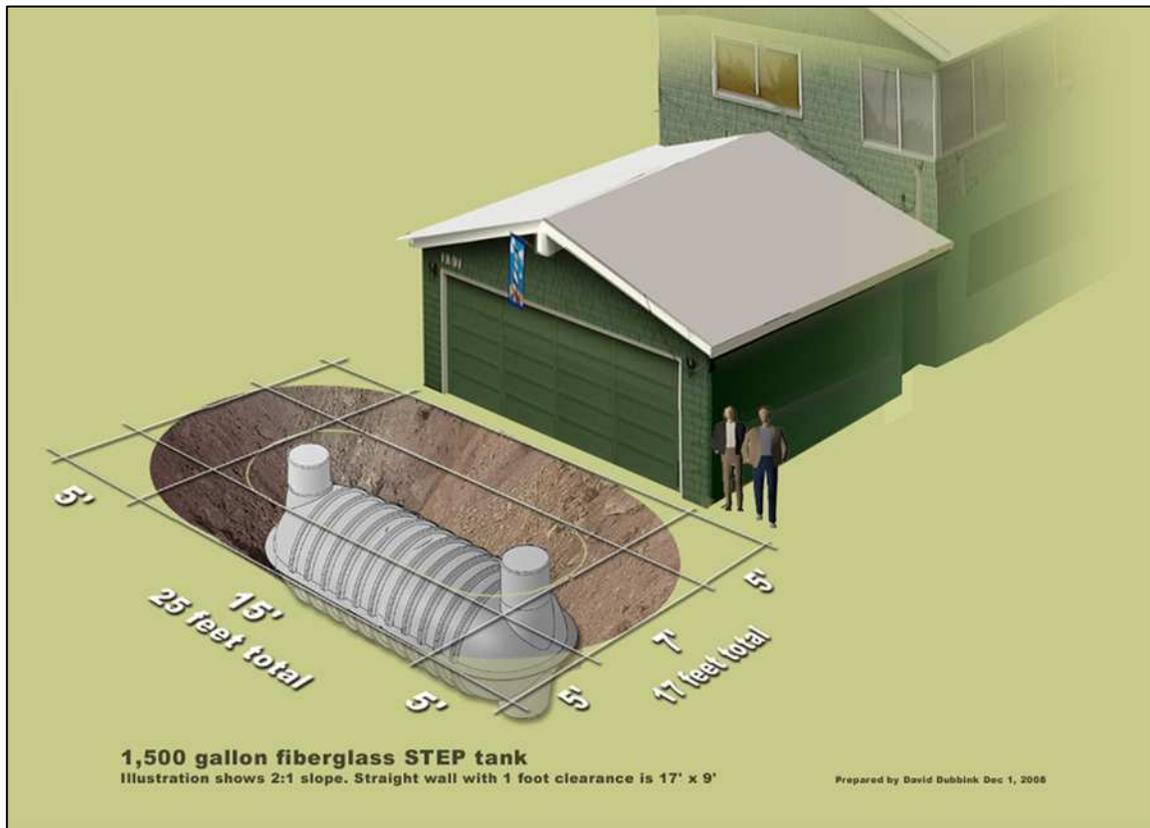
Figure 2: STEP Excavation
