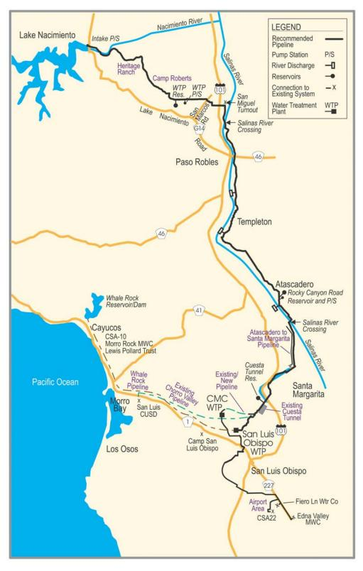
Figure 2-2 Schematic of Raw Water Option
