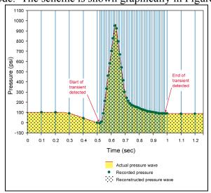
Figure 3 – TP-1 Data Recording Scheme
