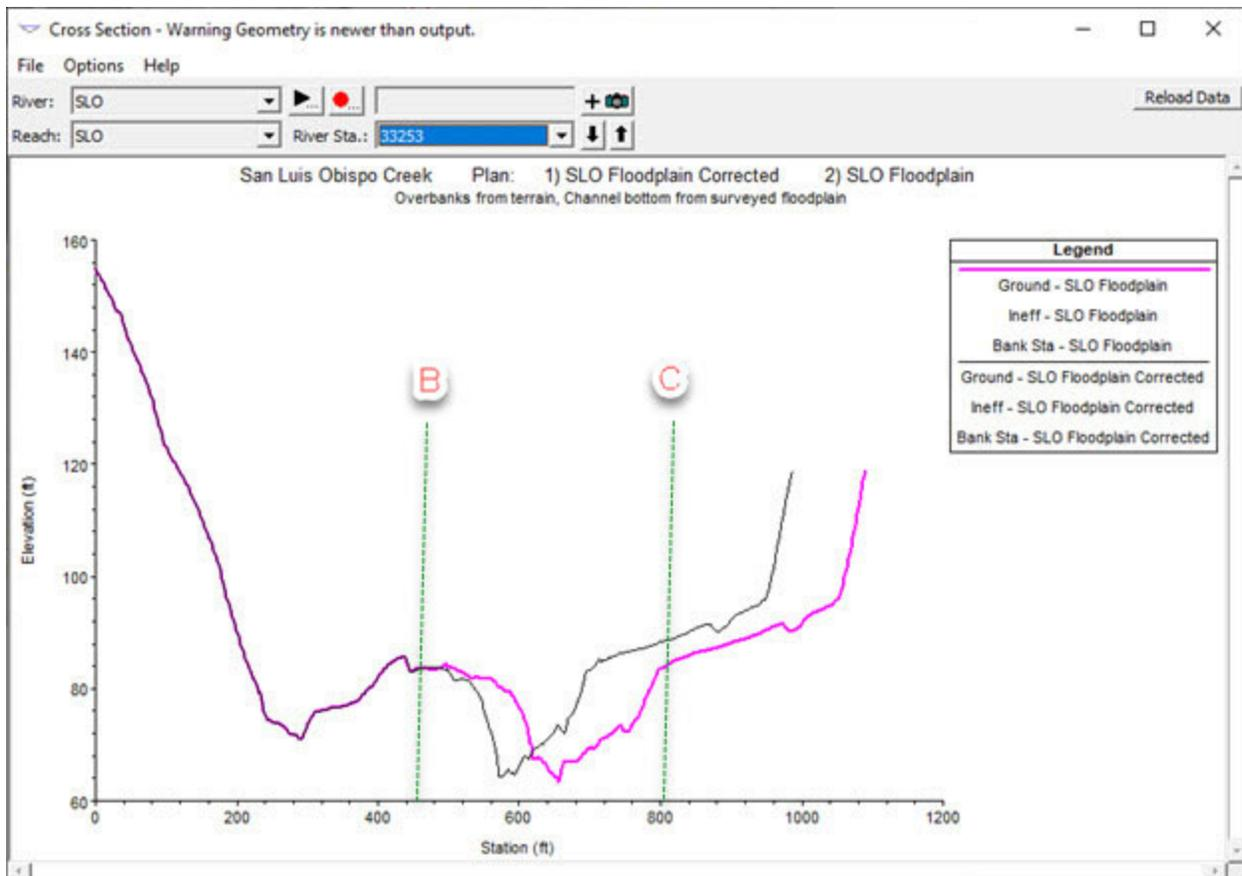
Figure 7. Comparison of RS 33253 cross section data between FEMA (magenta) and changed (black) with segment between B-C skewed 45 degrees
