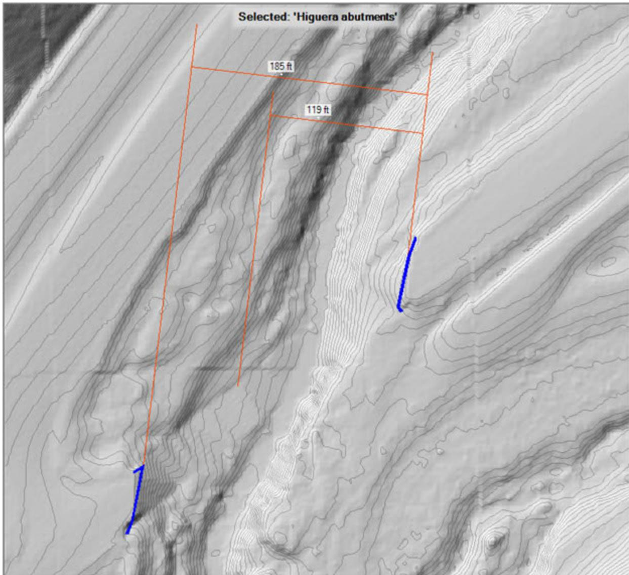
Figure 10. Comparison of the effective hydraulic openings between the FEMA geometry (119 ft) and the changed geometry (185 ft). Surveyed abutments shown in blue.
