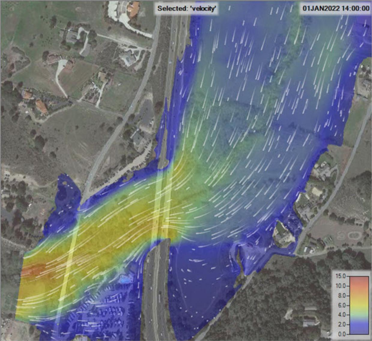
Figure 1. Flow pattern through Highway 101 bridges.
