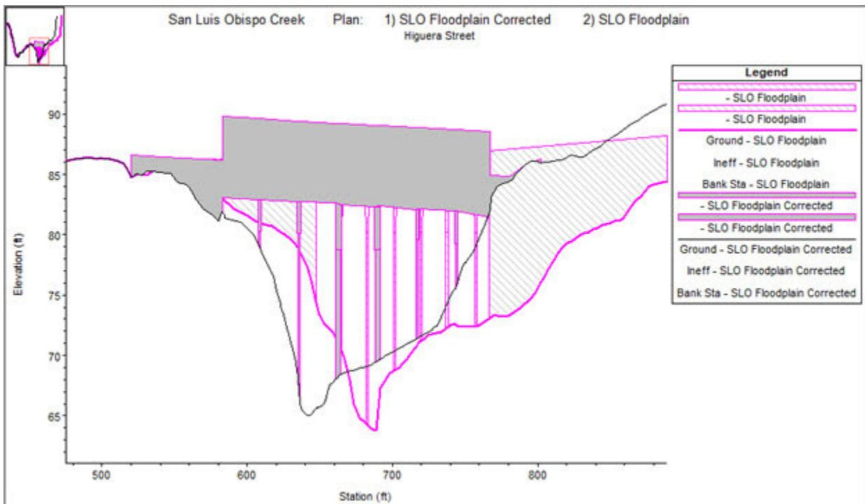
Figure 9. Comparison of the FEMA geometry to the changed geometry for the Higuera Street Bridge (RS 33278) zoomed in
