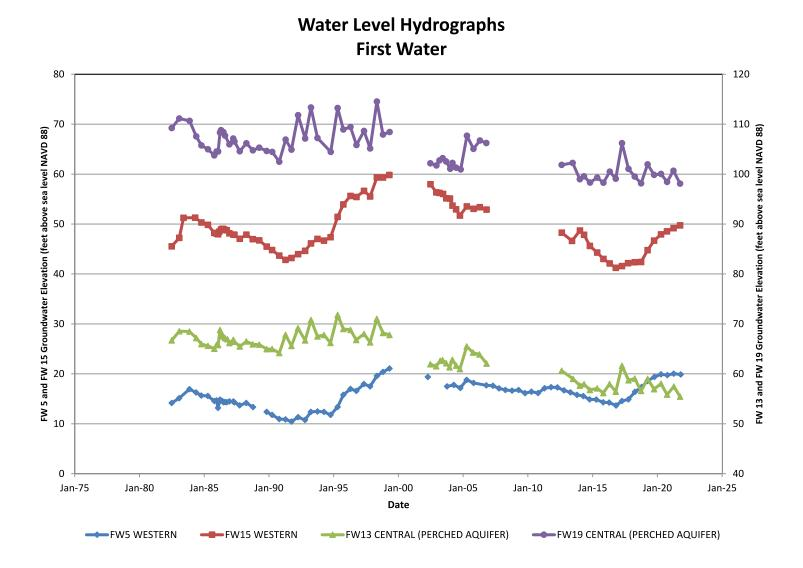
Figure 15 Water Level Hydrographs Perched Aquifer / First Water Los Osos Groundwater Basin 2021 Annual Report
