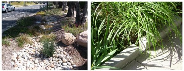
Examples of parkway/LID and curb cuts applications allowing for water infiltration.
