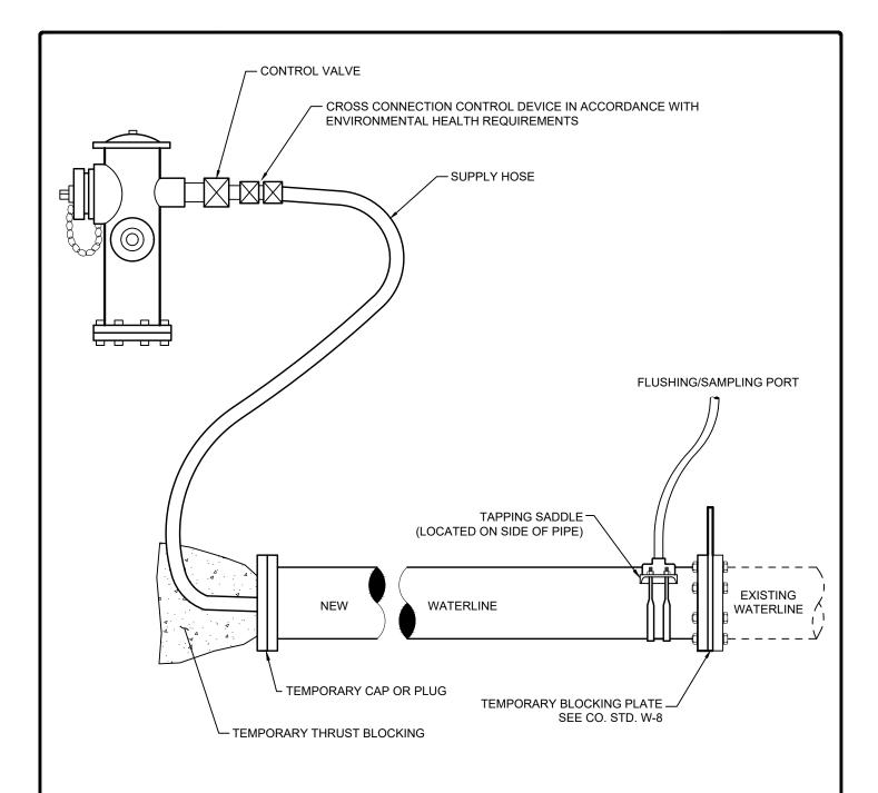
1. DIRECT CONNECTION TO THE EXISTING WATER SYSTEM SHALL NOT BE PERMITTED UNTIL THE NEW INSTALLATION HAS PASSED BACTERIA TESTING. MAINTAIN AIR GAP PER AWWA STD. C651.
