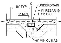
ADD SCORE LINE IN CONCRETE DIRECTLY ABOVE PIPE EDGES
