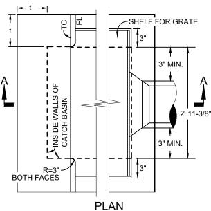
DEPARTMENT MAY REQUIRE A STAINLESS STEEL FRAME DESIGNED TO ACCEPT A "DrainPac™" STORM DRAIN FILTER INSERT, OR EQUAL.
