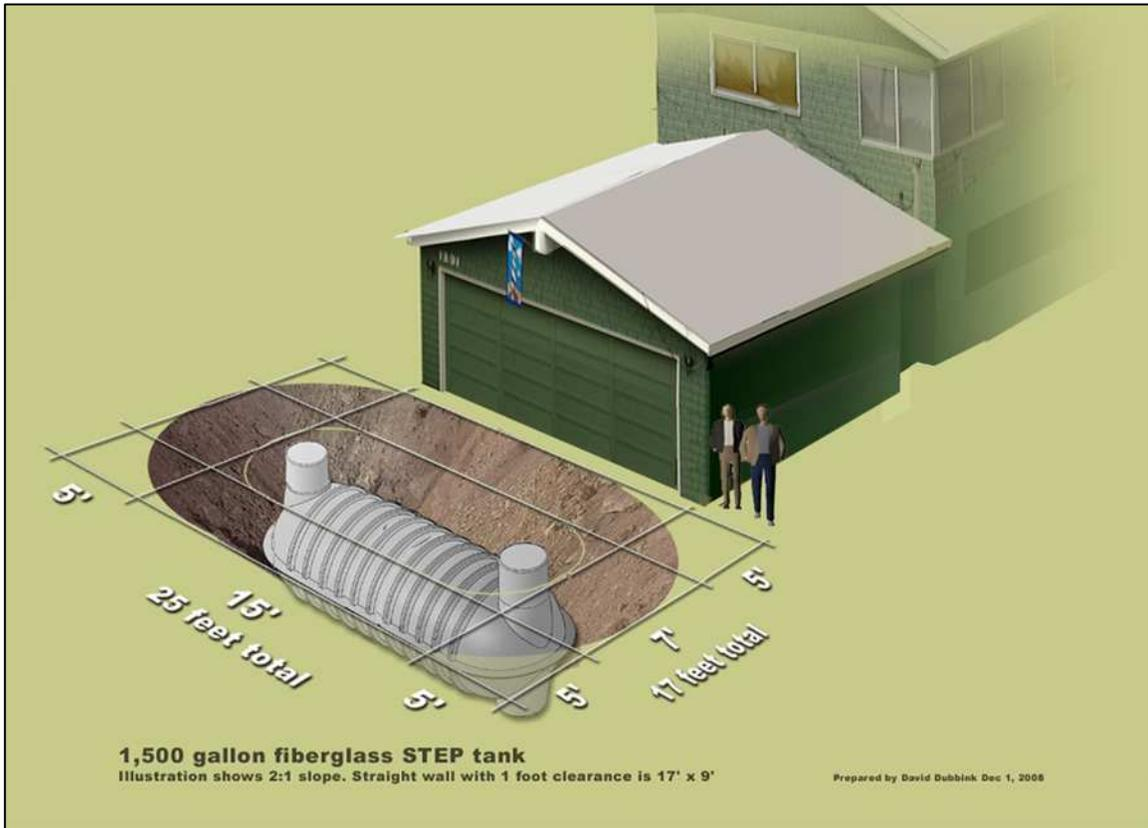
Figure 2: STEP Excavation
