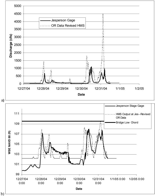
Figure 10. Jesperson Road Bridge a) discharge hydrograph b) water surface elevation hydrograph
