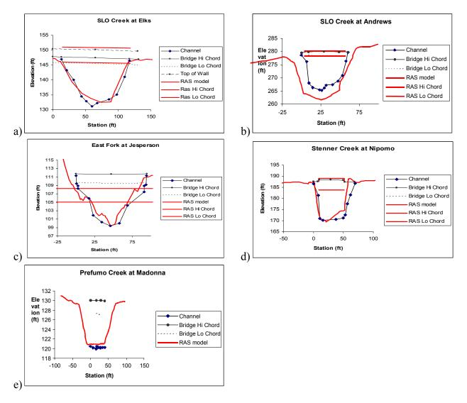
Figure 5. Cross-sections at County stage gage locations with red lines showing LIDAR data used for the existing hydraulic model and blue lines showing 2006 survey data, which was used to update the hydraulic model: a) Elks Lane Bridge over SLO Creek b) Andrews Street Bridge over SLO Creek c) Jesperson Road Bridge over East Fork of SLO Creek d) Nipomo Street Bridge over Stenner Creek e) Madonna Road Bridge over Prefumo Creek.
