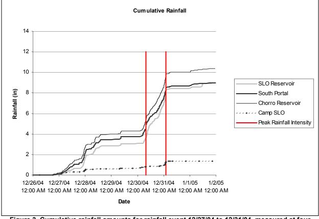
Figure 3. Cumulative rainfall amounts for rainfall event 12/27/04 to 12/31/04, measured at four County rain gages.
