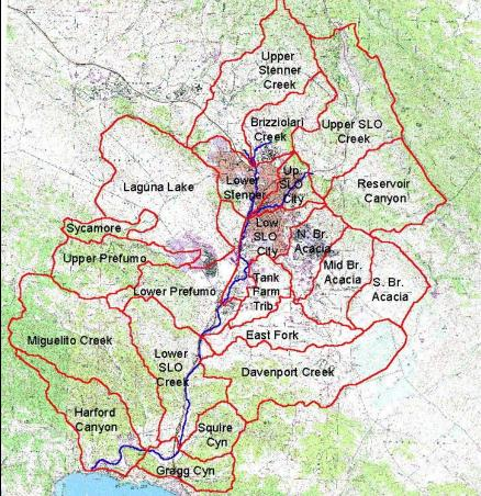
Figure 1. Hydrology model sub-basin delineation
