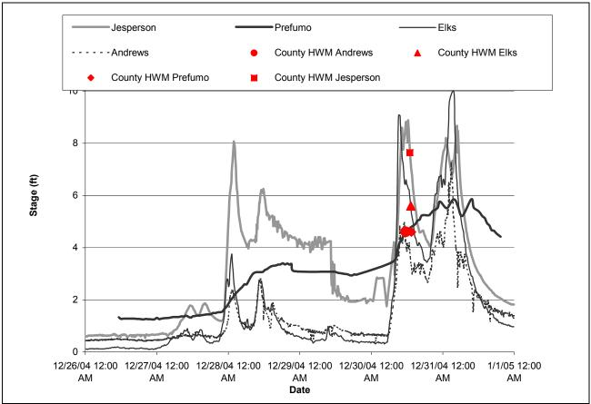
Figure 7. Stage gage output and corresponding County high water marks during the December 2004 storm.
