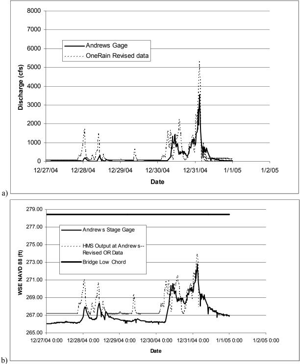
Figure 9. Andrews Street Bridge a) discharge hydrograph b) water surface elevation hydrograph
