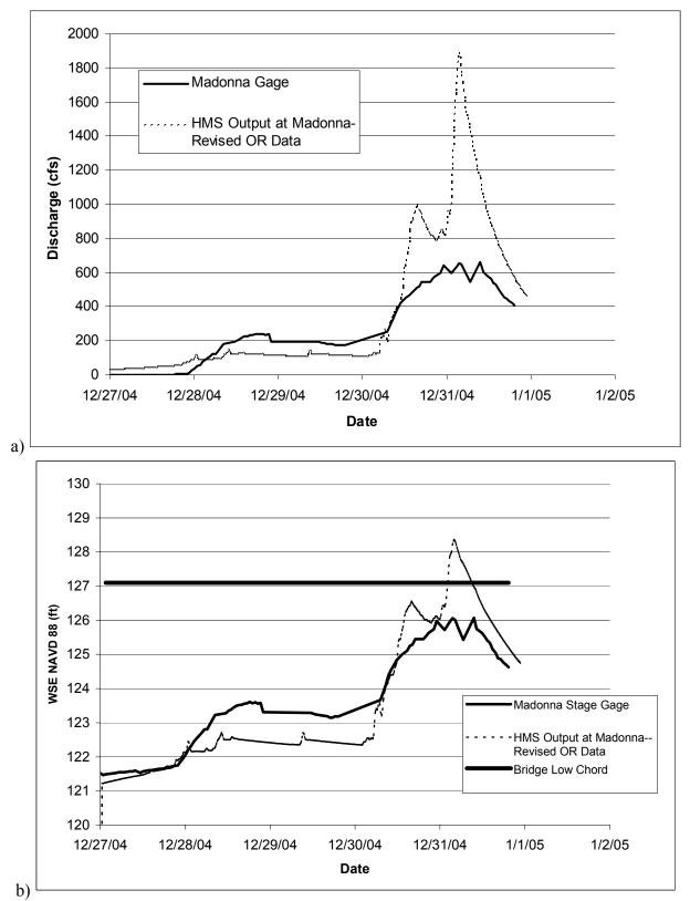
Figure 11. Madonna Road Bridge a) discharge hydrograph b) water surface elevation hydrograph
