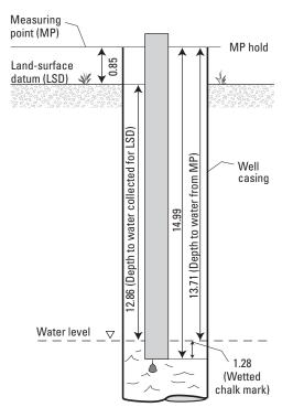
**Figure 1.** Water-level measurement using a graduated steel tape.
