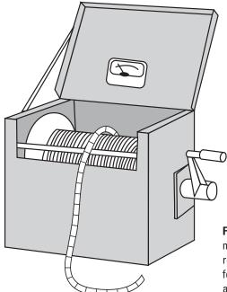
**Figure 2.** Older model electric tape, also known as "M-scope" marked at 5-foot intervals with clamped-on metal bands, has been replaced by newer, more accurate models. Technical procedures for this device are available from the procedures document archives.
