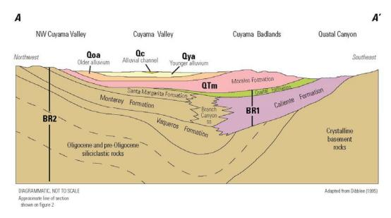
FIGURE 6: Stratigraphic Diagram of the Cuyama Valley Area
