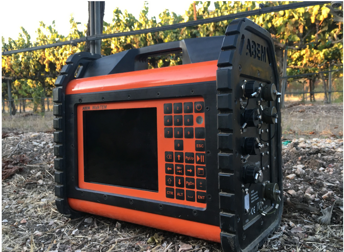
Figure 2 WalkTEM. The transmitter and the receiver is combined in one instrument that can be hand carried from site to site.
