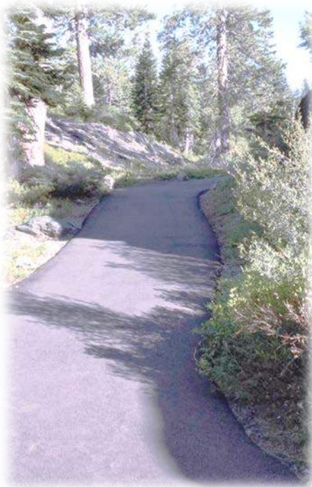
An 8-foot wide asphalt trail system surfaced with asphalt or decomposed granite is preferred over costly and fractured concrete sidewalk improvements
