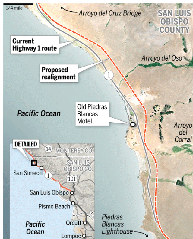
Figure 30: Sea-level rise may increase flooding of Highway 1 along the northern portion of the county. This map shows one proposed idea for relocating the highway in response to such risks.
