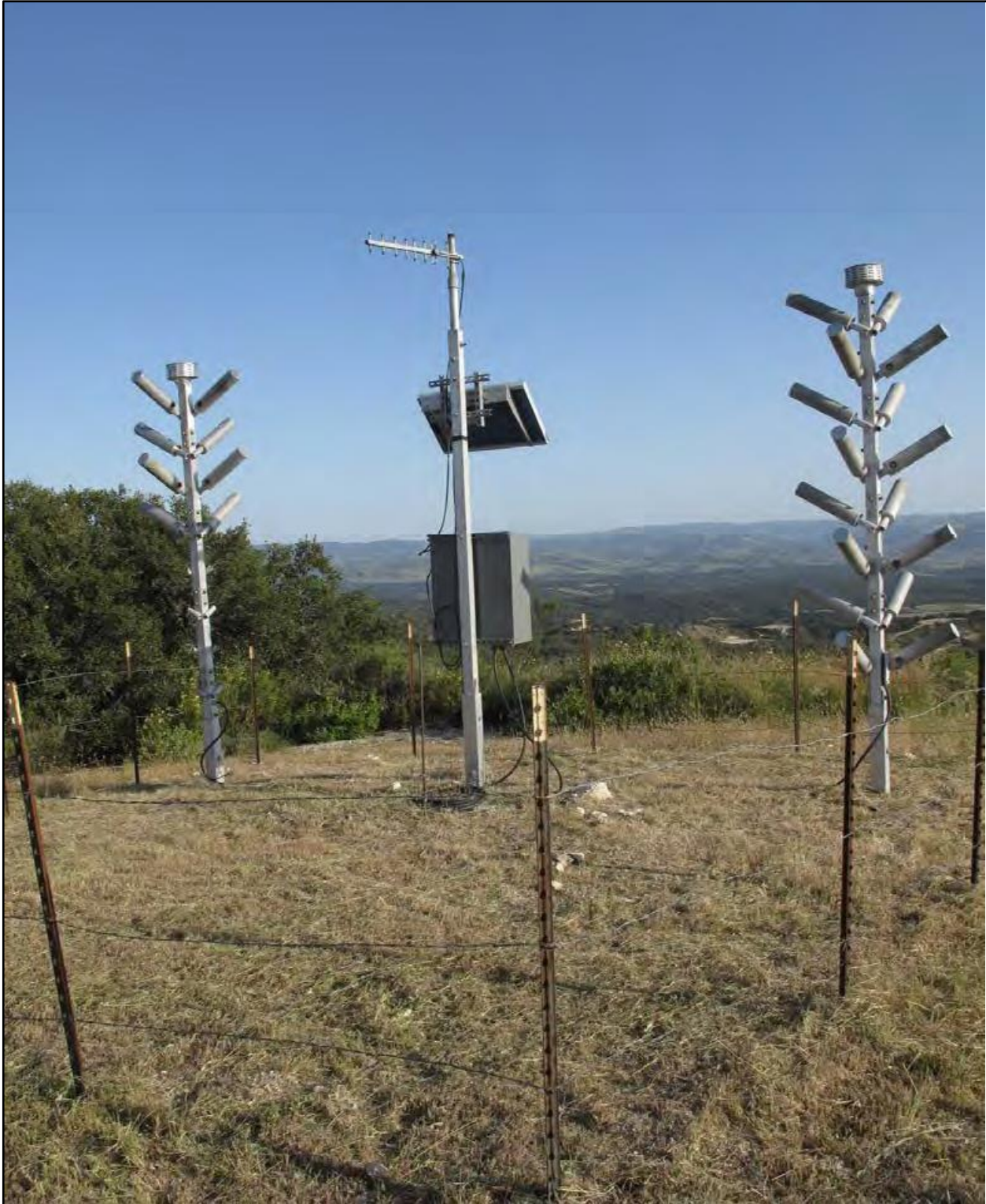
Figure 3 Typical ground seeding site. Note limited disturbance necessary, with the exception of vegetation maintenance.
