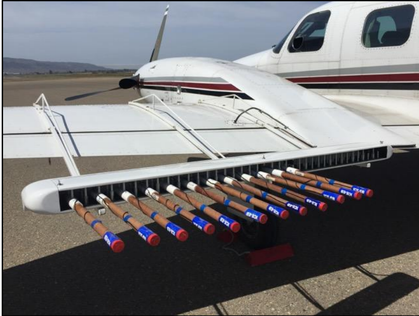
Figure 1. Typical cloud seeding aircraft with mounted flare rack.
