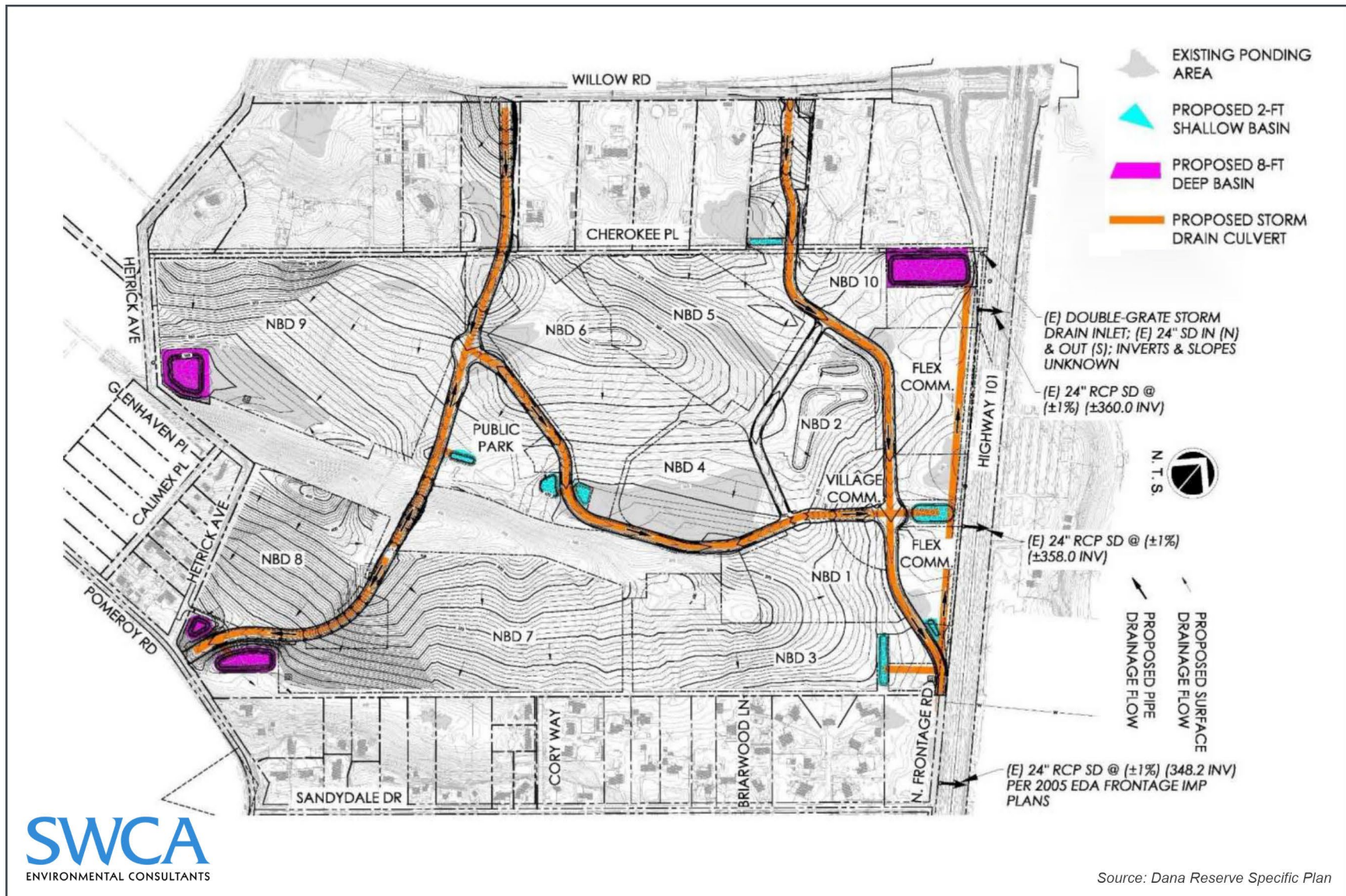
Figure 2-23. Proposed Stormwater Management Facilities.
