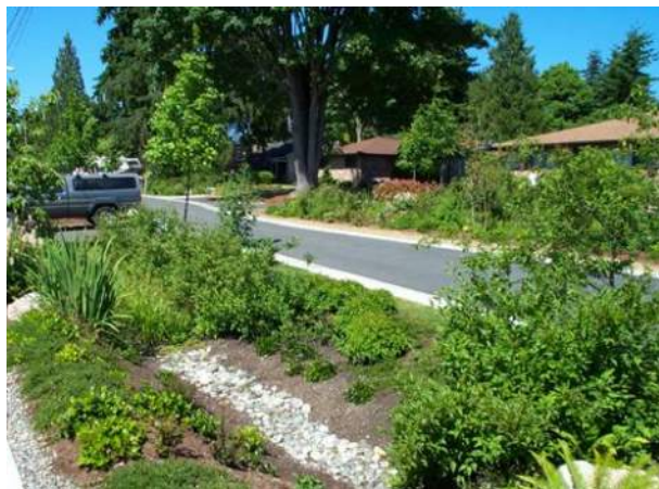
Parkway medians provide opportunities for decentralized biofiltration and retention.
