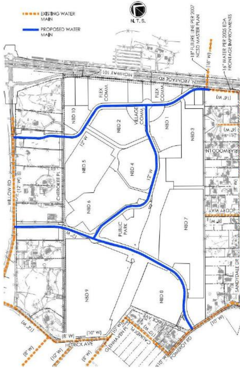
Exhibit 5-1: Proposed Water Backbone Infrastructure
