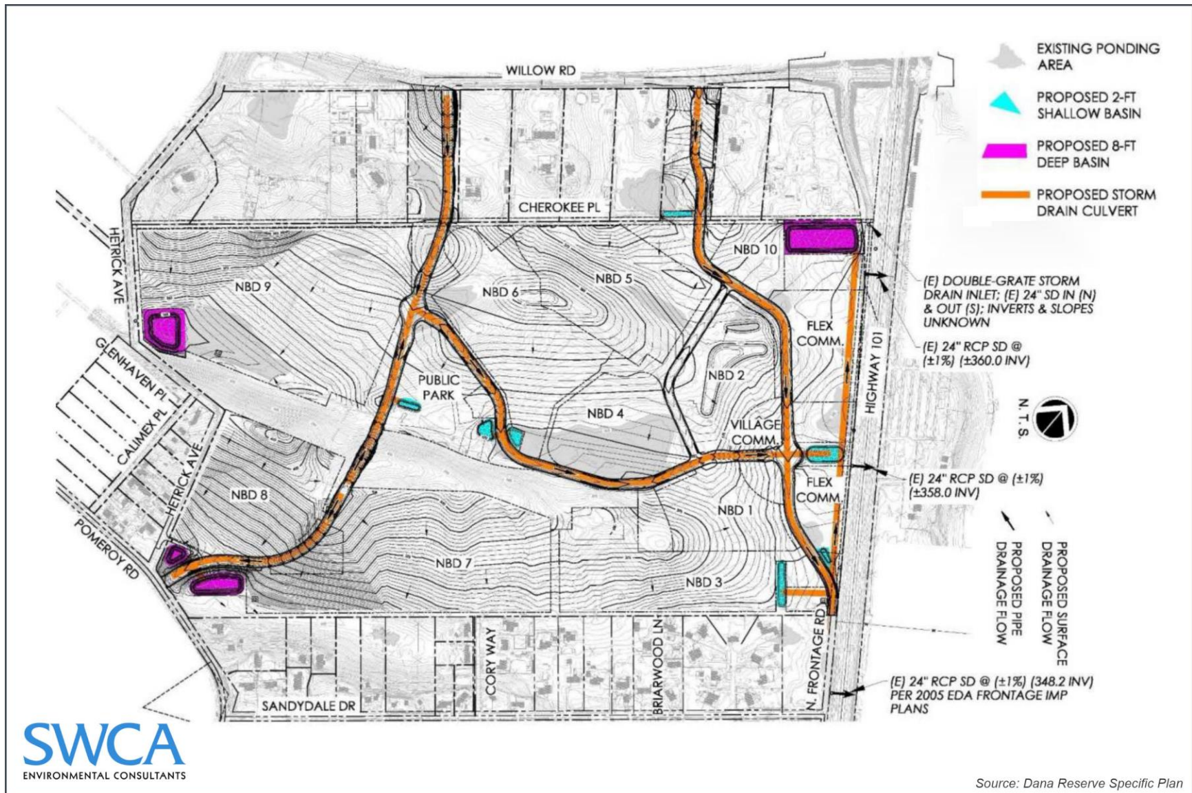
Figure 4.10-3. Proposed Stormwater Management Facilities.
