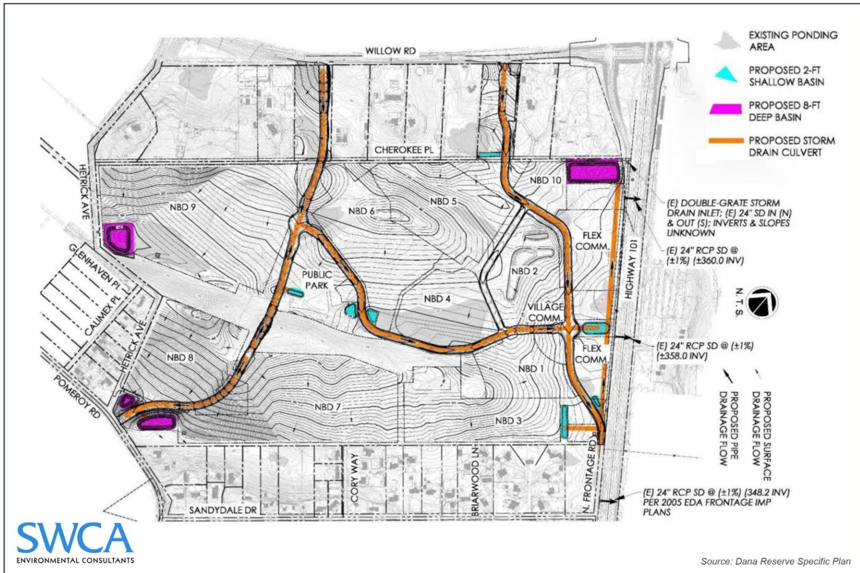
Figure 2-23. Proposed Stormwater Management Facilities.
