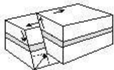
(f) left-lateral reverse fault (left-oblique reverse fault)
