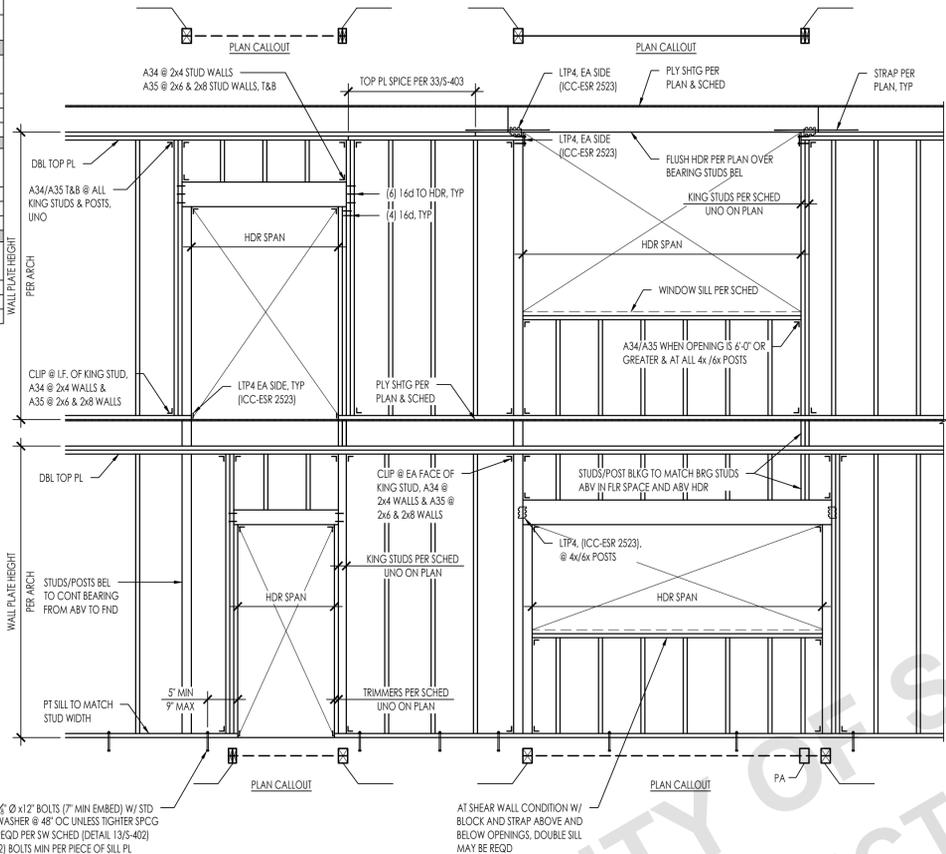
EXTERIOR WALL / INTERIOR WALL BEARING WALL FRAMING
