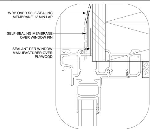
**12 DETAILED JAMB FLASHING**
