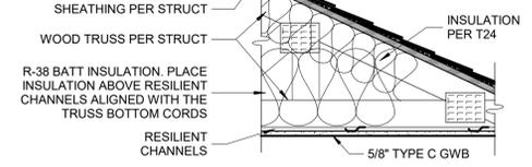
R-38 BATT INSULATION. PLACE INSULATION ABOVE RESILIENT CHANNELS ALIGNED WITH THE TRUSS BOTTOM CORDS
