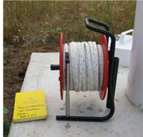
Well Sounding Probe
