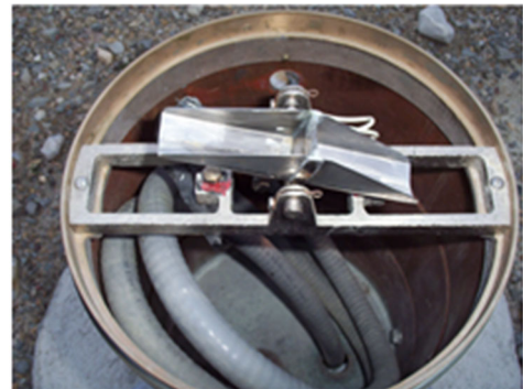
Real-Time Tipping Bucket Rain Gauge
