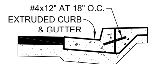
8 SIDEWALK WIDENING DETAIL NTS
