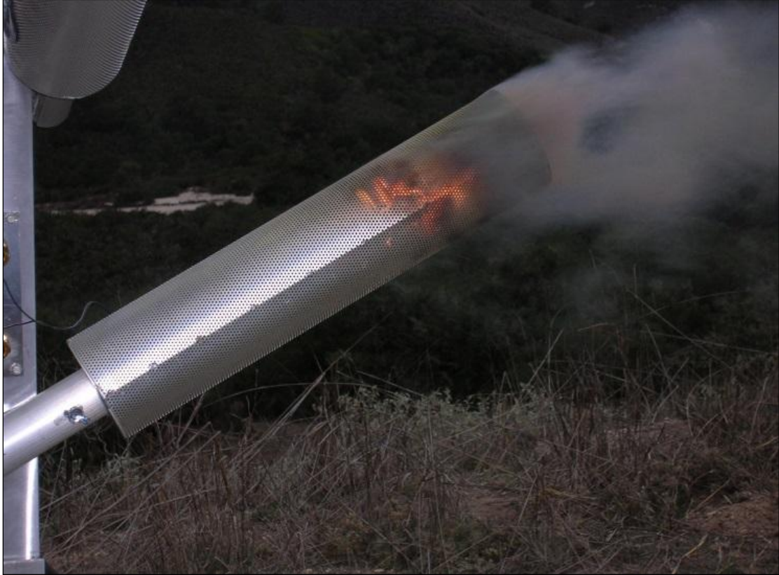
Figure 5.7 Flare Burning Inside Spark Arrestor
