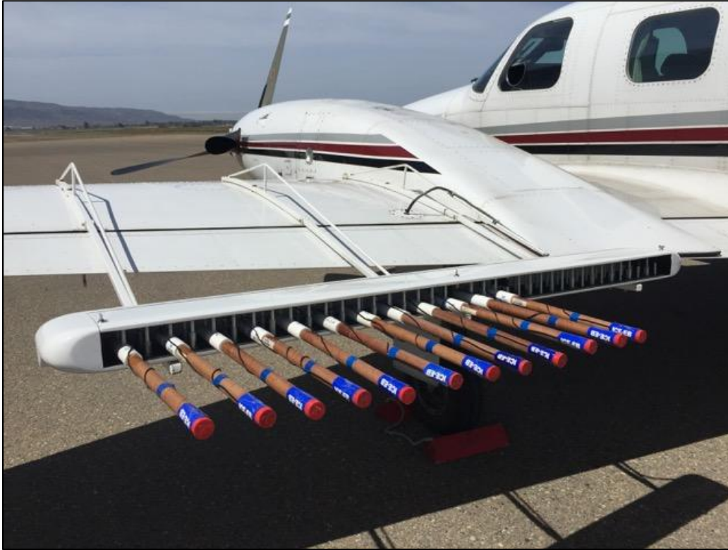
Figure 5.2 Cheyenne II Cloud Seeding Aircraft with End Burning Flare Racks
