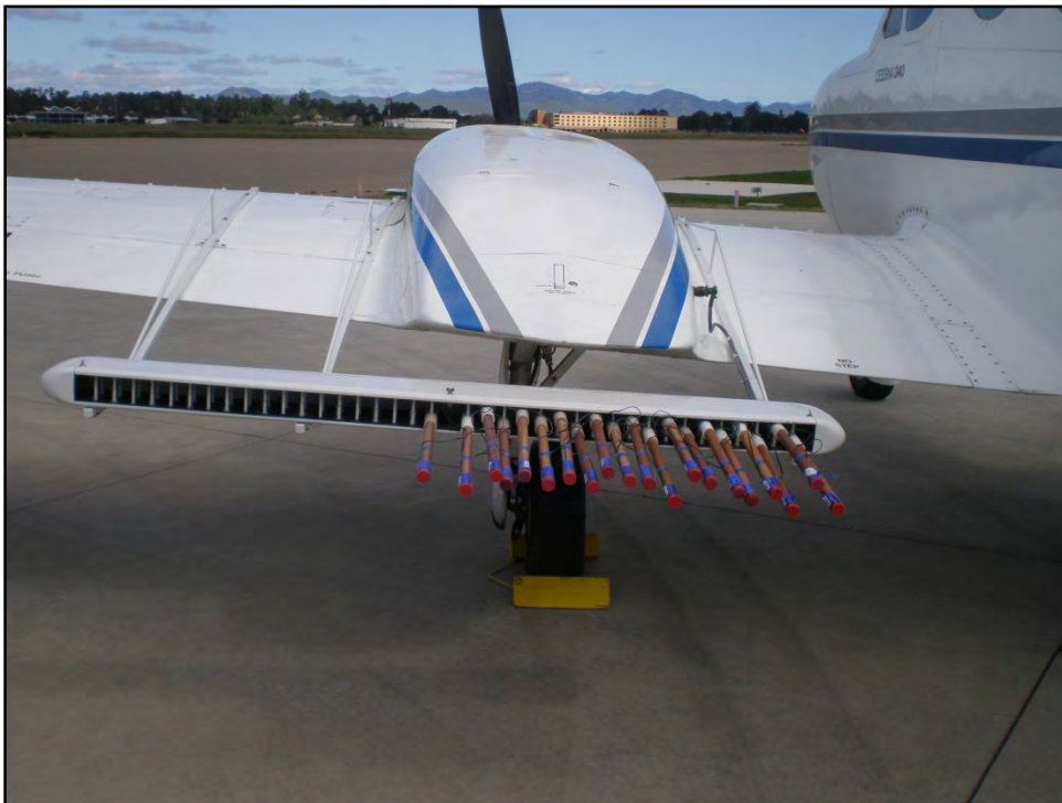
Figure 5: Flare Rack Mounted to Cessna 340 Aircraft
