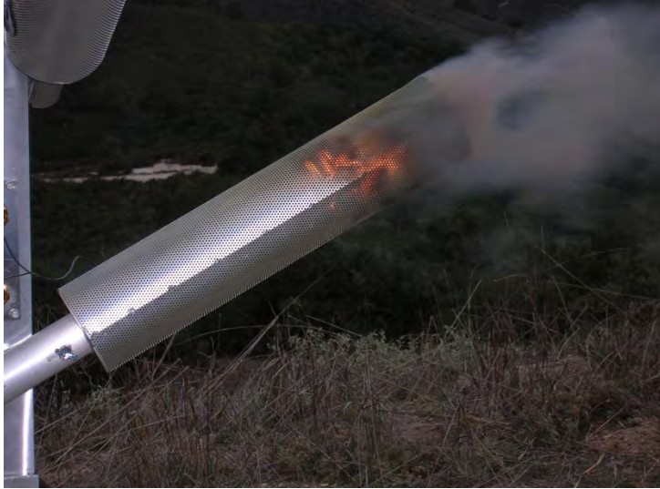
Figure 3: Flare Burn with Spark Arrestor
