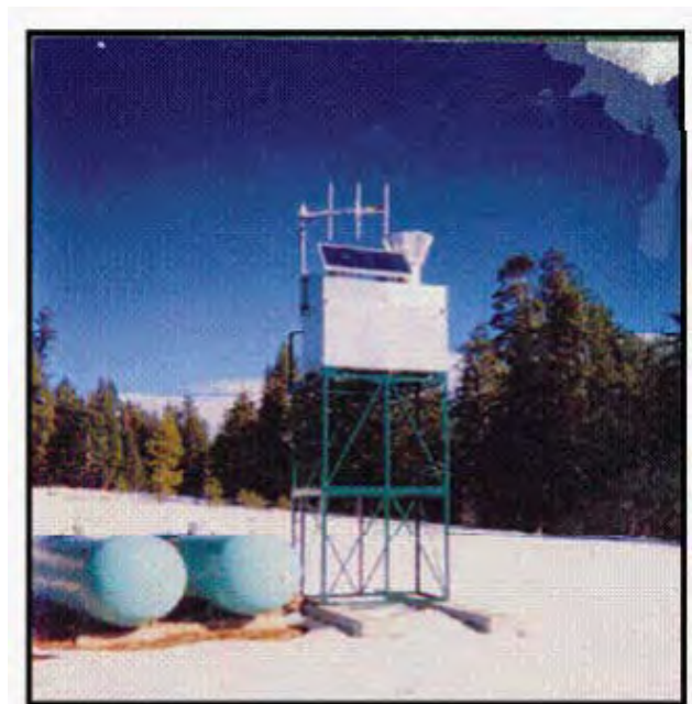
Photo Image of ground-based seeder. Image courtesy of Pacific Gas and Electric Company
