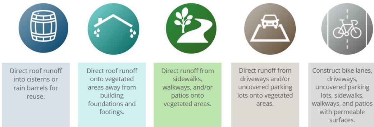
463 Figure 5: Runoff reduction measures, PR#1
