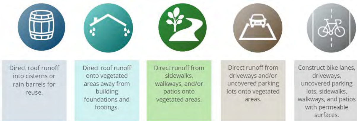
Figure 5: Runoff reduction measures, PR#1.
