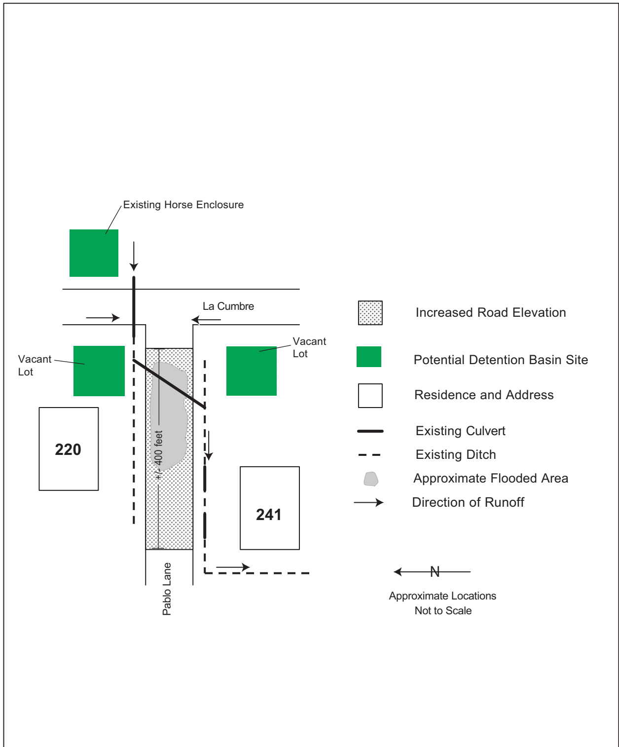
Nipomo Mesa Drainage and Flood Control Study Proposed Project 2 Schematic Pablo Lane and La Cumbre
