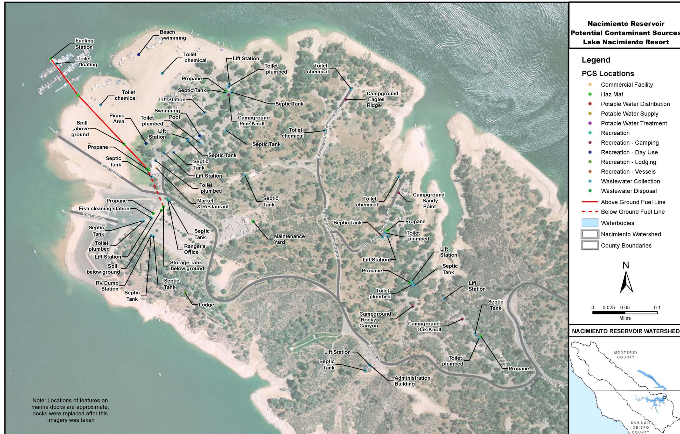
Figure 80: Lake Nacimiento Resort Fuel Line to Docks
